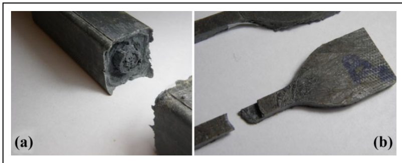
Figure 9. Analyzed specimens: extruded bars (a) and type ASTM D638-14 normative (b). ASTM: American society for testing and materials.
