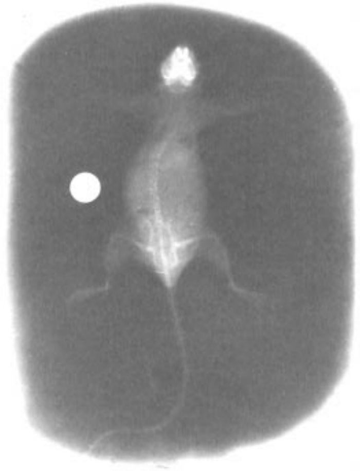
Fig. 8. X-ray image of a mouse taken with a single shot of the DPF at one meter to focus, the detailed structure of the specimen can be seen.
