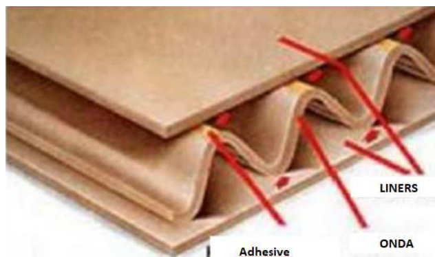
Figure 1. Location of a wave paper in corrugated cardboard.
