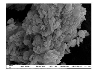
Fig. 14 SEM image of spent Zn-Nit salt after three reaction uses at 100  $^\circ\text{C}.$
