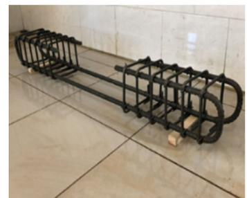
FIGURE 1 Geometry, reinforcement details and loading scheme of reinforced concrete beams with  $\rho_s = 0.5\%$  and  $\rho_s = 1.2\%$
