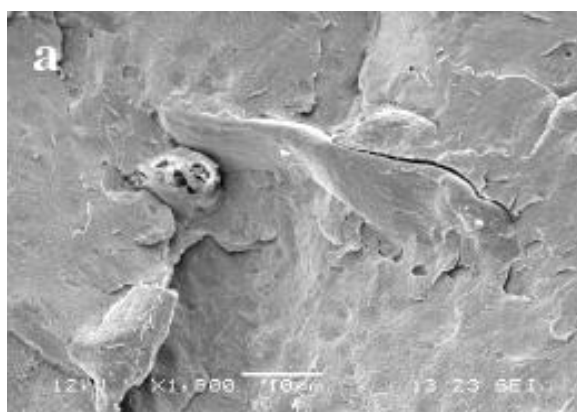
Figure 8. SEM micrographs of (a) PS/Cell and (b) PS/Oat composites.
