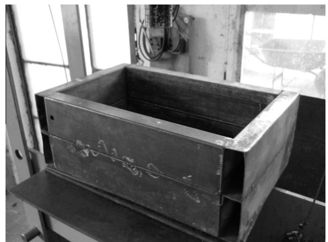
Fig. 6. Mold made with iron sheets.
