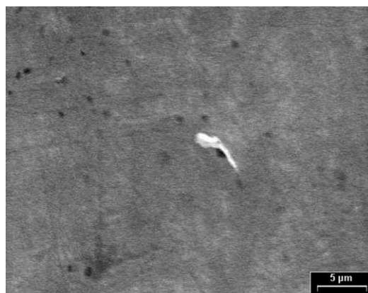
Fig. 9. Stabilized Zn surface at RH 0.33% and 21 °C—time of reaction 3600 s.
