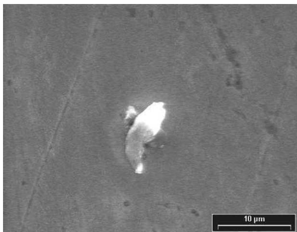
Fig. 10. Stabilized Zn surface at RH 0.33% and 21 °C—time of reaction 9000 s.
