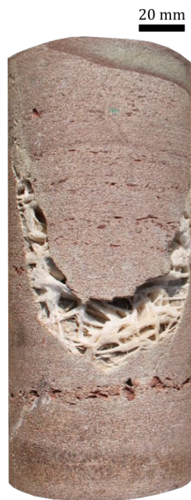
Figure 1. Photograph of a section of 78 mm-diameter, cylindrical sandstone core (from the Buntsandstein unit) taken from the Soultz-sous-Forêts (France) EPS-1 exploration borehole, a borehole fully cored from a depth of 930 m to a depth of 2227 m in 1990-1991 (see 5-7 for information on the Soultz-sous-Forêts drilling project). The sandstone core, red/green in color, was taken from a depth of 1374 m and contains a 1-2 cm-wide fracture (in the center of the core). The fracture is partially filled with barite crystals (white in color) that have precipitated from the circulating geothermal fluids.
