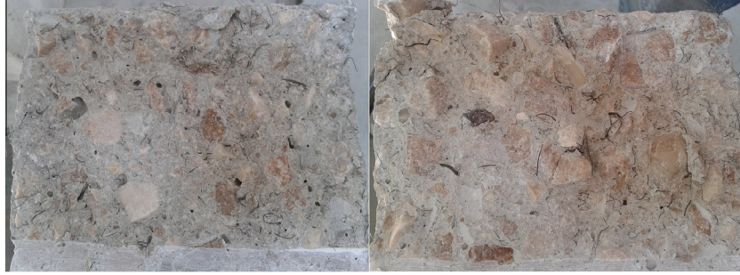
Fig. 15. Observed distribution of fibres at crack section for one of the specimens (mixture RSFRC 100-05).
