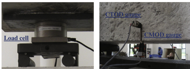
Fig. 12. Disposition of the instrumentation for the four-point bending tests.
