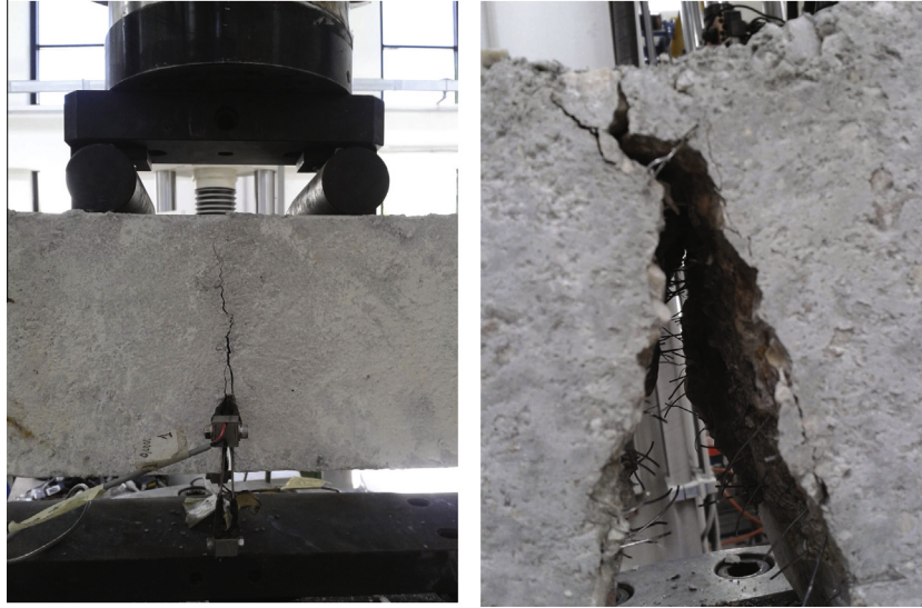
Fig. 13. Cracked configuration after the 4 PB test of HRSFRC notched beams.
