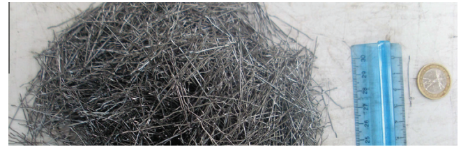
Fig. 9. Industrial fibre types FS7 [32] employed for the HIRSFRC.
