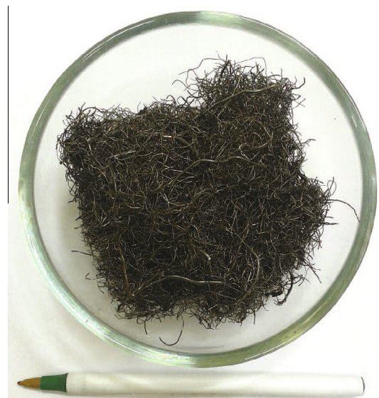
Fig. 1. Recycled Steel Fibres employed for the HIRSFRC.
