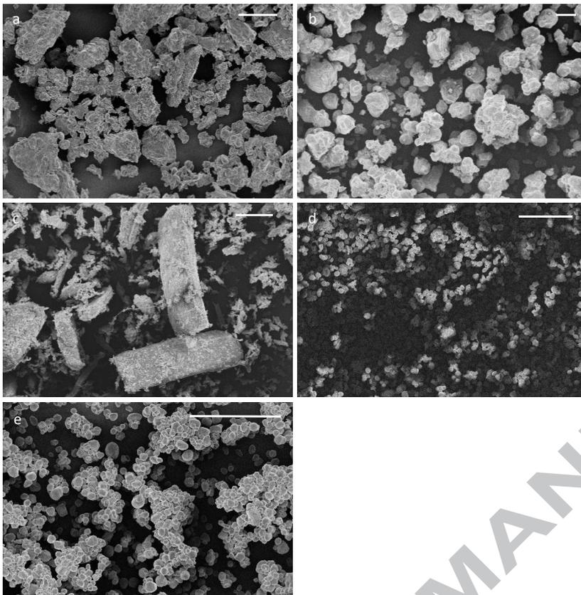
**Figure 3. Microphotographs of SEM. a) wheat flour, magnification 150x; b) inulin, 80x; c) oat fiber, 144x; d) RSII, 200x and e) RSIV, 350x. Barr: 100  $\mu$ m.**
