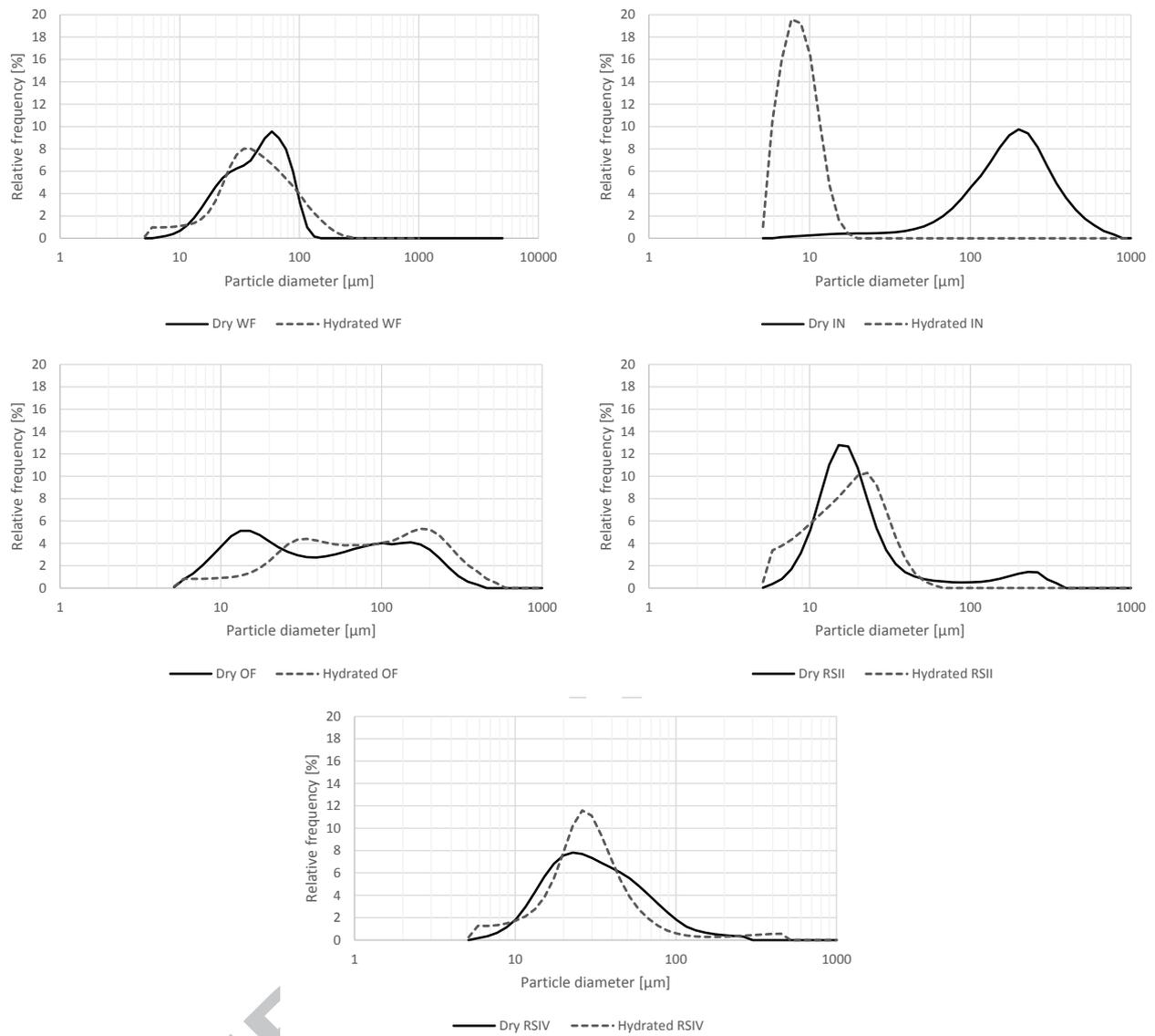
Figure 4. Particle size distribution of dry and hydrated samples. WF: wheat flour; IN: Inulin; OF: Oat fiber; RSII: Resistant starch II; RSIV: Resistant starch IV.
