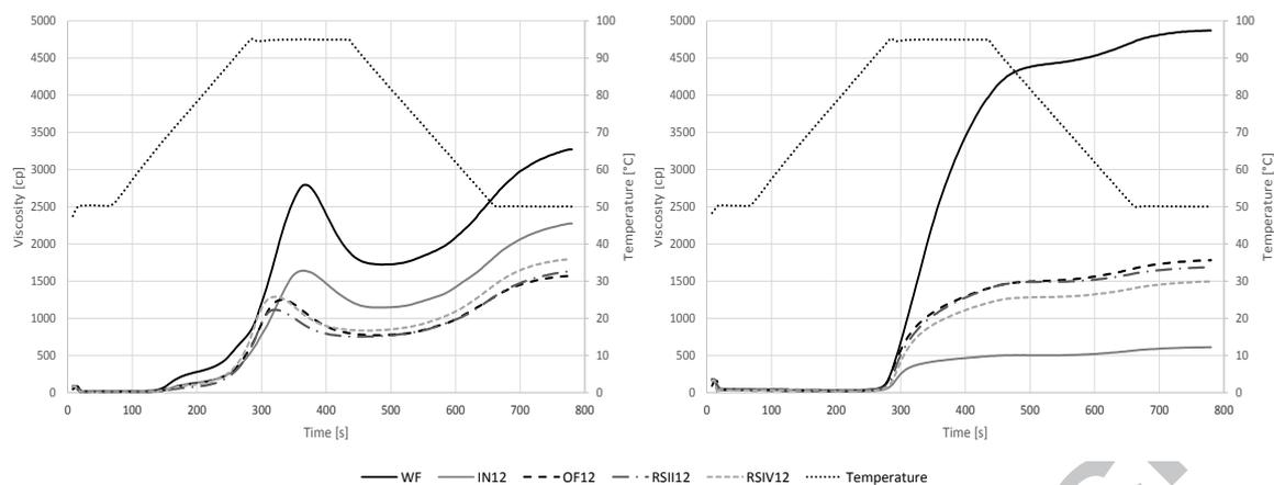
**Figure 2. Effect of fiber addition on the pasting profile using water (a) and 50% sucrose solution (b) as a solvent. WF: wheat flour; IN: Inulin; OF: Oat fiber; RSII: Resistant starch II; RSIV: Resistant starch IV. 12 refer to fiber incorporation level.**
