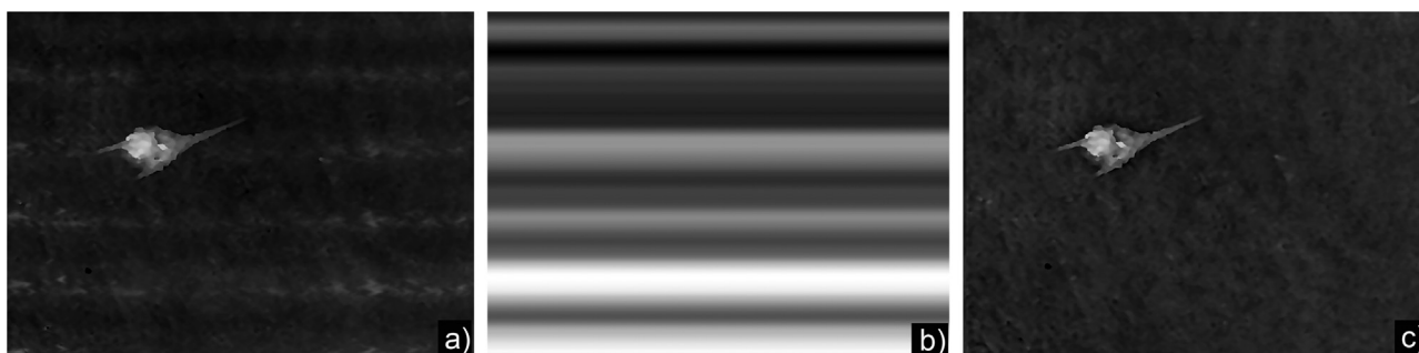
Fig. 5. : a) Original unwrapped phase map, b) Filter Matrix, c) Corrected unwrapped phase map.
