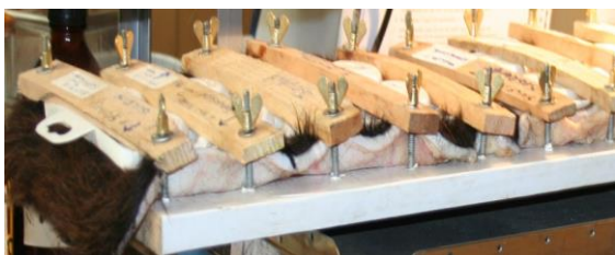
Fig.1. - Permeability assay: plastic plates holding bovine skin
