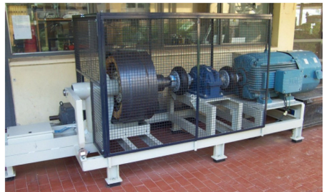
Fig. 7 Generator mounted on test bench
