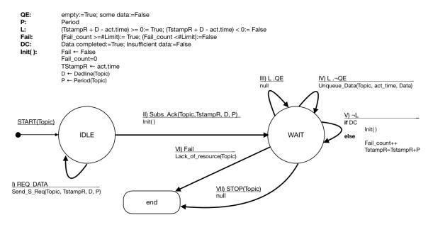
Figure 6. FSM representing the behavior of the processor.
