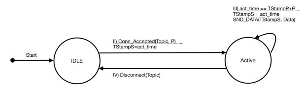
Figure 5. Finite state machine (FSM) representing the behavior of the terminals.
