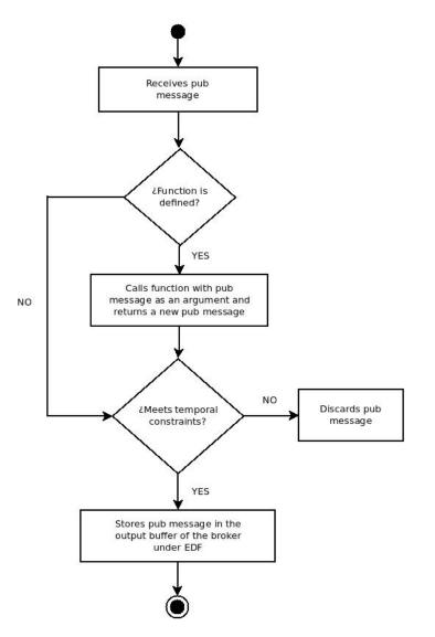
**Figure 8.** High-level activity diagram of a publication message processing of the intelligent real-time agent (IRTA).
