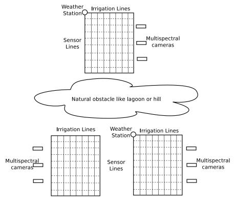
Figure 18. Sensors deployment in a hypothetical precision agriculture (PA) scenario.
