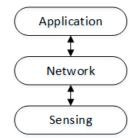
Figure 1. Layered structure of an Internet-of-Things (IoT) interaction scenario.
