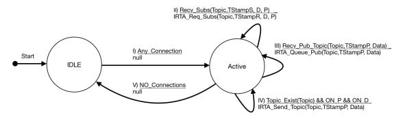
Figure 7. State machine diagram for broker.
