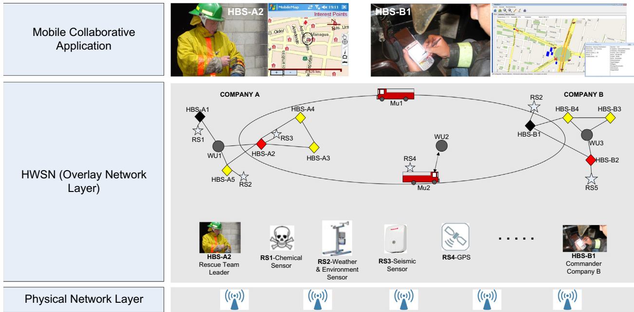
Fig. 5. Basic architecture of a collaborative system supported by HWSN.
