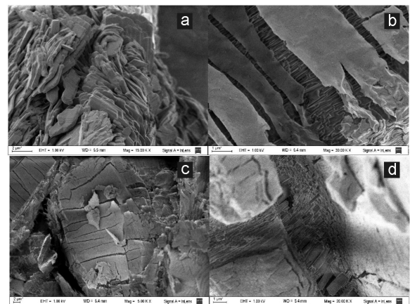
Figure 3. SEM images. a: fluconazole raw material; b: crystals from 10 % propylene aqueous solutions; c: crystals from 10 % Transcutol P® (TCL) aqueous solutions; d: magnified inner part of the hydrate crystal from 10 % TCL aqueous solutions.
