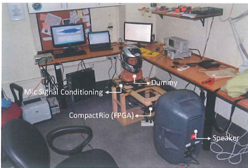
Fig. 2 Identification and control experimental setup.
