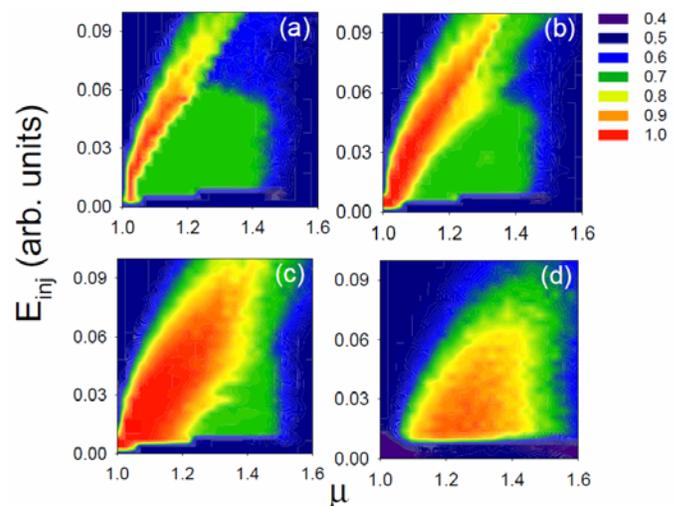
Fig. 4 (Color online) Success probability computed with 80/20 criterion, as a function of the injected field amplitude,  $E_{inj}$ , and the pump current parameter,  $\mu$ .  $D=10^9 \text{ ns}^{-1}$  (a),  $10^5 \text{ ns}^{-1}$  (b),  $10^3 \text{ ns}^{-1}$  (c), and  $D=10^1 \text{ ns}^{-1}$  (d); other parameters are as in Fig. 2.
