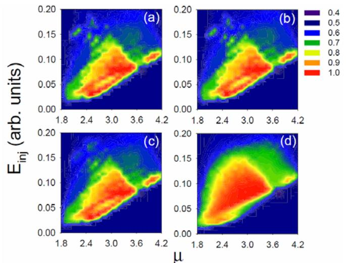
Fig. 9 (Color online) Success probability with  $y$  polarized injection as a function of the pump current parameter,  $\mu$ , for noise strength:  $D=10^{-9}$  ns $^{-1}$  (a),  $10^{-5}$  ns $^{-1}$  (b),  $10^{-3}$  ns $^{-1}$  (c), and  $10^{-1}$  ns $^{-1}$  (d).  $T=5$  ns and  $\Delta\omega_c=150$  rad GHz, other parameter as in Fig. 7.
