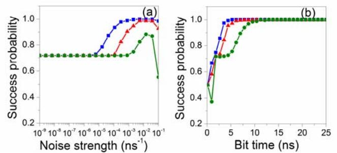
Fig. 3 (Color online) Success probability a function of the noise strength  $D$  (a) and of the bit time  $T$  (b) using the criteria 70/30 (squares), 80/20 (triangles), and 90/10 (circles). In (a)  $T=4.5 \text{ ns}$ , in (b)  $D=10^3 \text{ ns}^{-1}$ , other parameters are as in Fig. 2.
