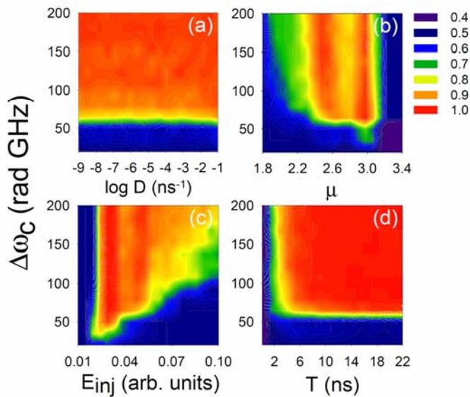
Fig. 10. (Color online) As Fig. 5 but with  $y$  polarized injection. When the parameters do not vary they are:  $\mu=2.5$ ,  $E_{inj}=0.05$ ,  $T=5$  ns, and  $D=10^2$  ns $^{-1}$ .
