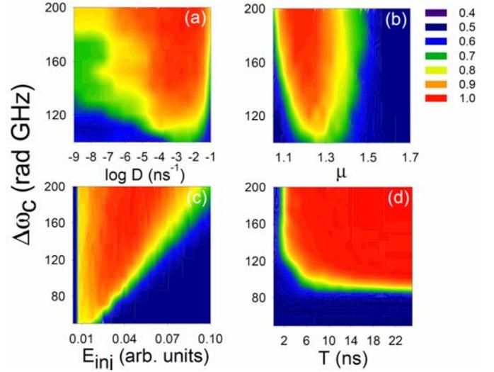
Fig. 5 (Color online) Success probability for  $x$  polarized injection, as a function of the detuning variation,  $\Delta\omega_c$ , and the noise strength,  $D$  (a); the pump current parameter,  $\mu$  (b); the injected field amplitude,  $E_{\text{inj}}$  (c) and the bit time  $T$  (d). When the parameters do not vary, they are  $D=10^{-3} \text{ ns}^{-1}$ ,  $E_{\text{inj}} = 0.05$ ,  $\mu=1.2$ ,  $T = 4.5 \text{ ns}$ ; other parameters are indicated in the text.
