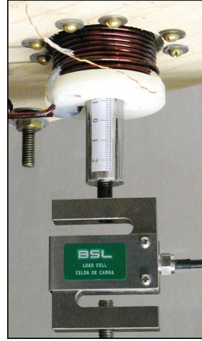
Fig. 10. Setup used to characterize the pull/push actuator strength for different displacements and current amplitudes. The coil was fixed to a rigid wooden platform, while the load cell was fixed to an optical table.
