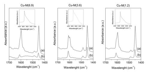
Fig. 9. FTIR of pyridine adsorbed on the samples modified with different copper contents, after desorption at 100 °C (a) and 200 °C (b). Inserted in spectrum of each sample is the region of OH before pyridine adsorption.
