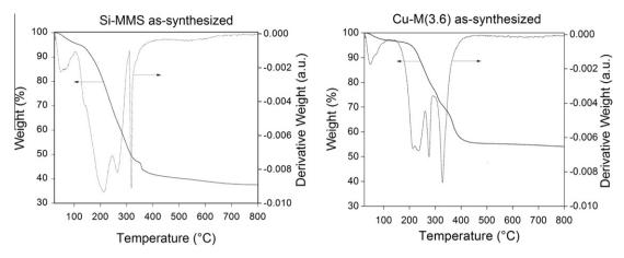
Fig. 5. TGA curves and derivatives of Si-MMS and Cu-M(3.6) as-synthesized samples.
