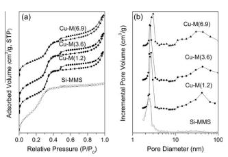
**Fig. 2.** N<sub>2</sub> adsorption/desorption isotherms and pore size distribution of the samples prepared with different copper contents.
