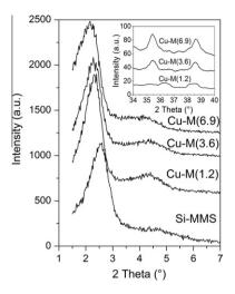
Fig. 1. XRD patterns of the samples prepared with different copper contents.
