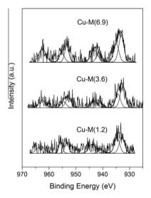
**Fig. 8.** Cu 2*p* core level photoelectron profile of the samples modified with different copper contents.
