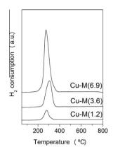
Fig. 7. TPR profiles of the samples modified with different copper contents.
