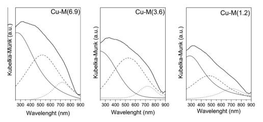
**Fig. 6.** UV–Vis diffuse reflectance spectra of the samples modified with different copper contents; experimental spectra, thick solid lines; decomposed contributions, thin lines; assignments: – isolated  $Cu^{\delta^+}$ , – oligomerics  $[Cu^{\delta^+}...O^{\delta^-}...Cu^{\delta^+}]_n$  species, CuO bulky oxides.
