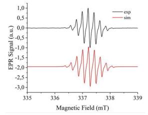
**Figure 3** Experimentally obtained and simulated EPR spectra after the insitu oxidation of **4**<sup>Dip</sup> with AgOTf.
