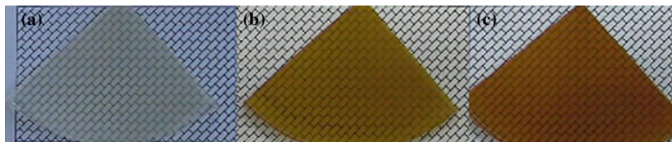
Fig. 1 Visual aspect of GTA cross-linked gelatin films a 0 wt% GTA, b 0.5 wt% GTA, c 1 wt% GTA
