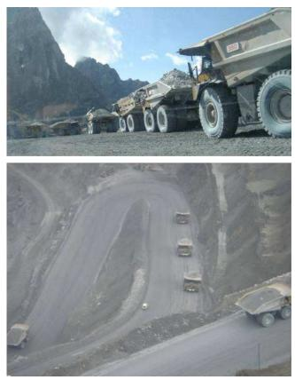
Fig. 2. Two areas of a mine that have different expected meaning for vehicle operators (different context meaning): (a) A dumping area where trucks park close together and (b) A haul road where vehicles must maintain separation of at least 50 m.
