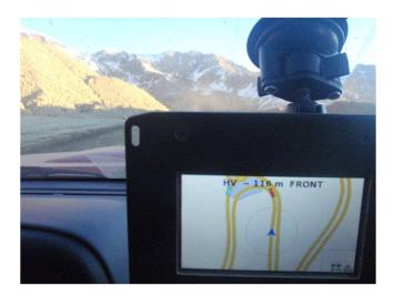
Fig. 10. The operator interface provides situation awareness information to the driver. There are two vehicles displayed on the screen that outside the operator's line of sight. An area of interest is shown at the top of the screen representing a large intersection.
