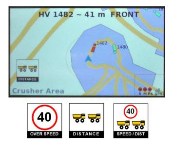
Fig. 11. Display implementation currently installed in mining vehicles. The context area name can be seen in the bottom left of screen. Several warning icons representing breaches of the rules are presented.
