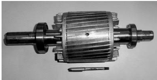
Fig. 13. Rotor with a broken bar.
