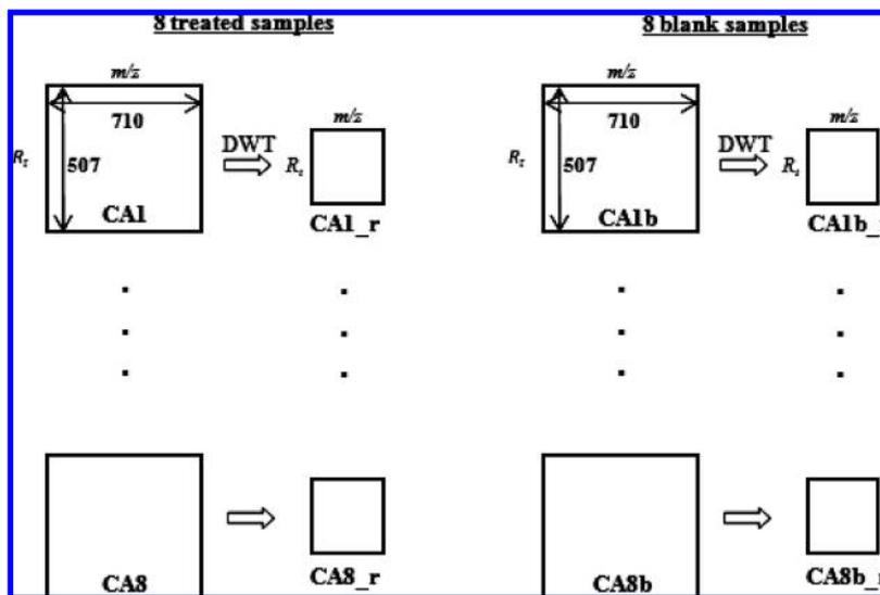
**Figure 1.** Sets of data matrices obtained during the analysis of samples treated and nontreated with pesticide. Both kinds of samples (treated and blank) were picked in 8 nonconsecutive days after the treatment of “Rambo” tomato plants with carbofuran. All these matrices were compressed by applying the DWT technique.
