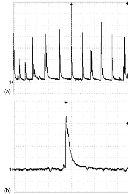
Figure 7. (a) Typical current signal for the plasma sheet regime; \Delta V = 26 kV; gas: dry air; H = 0 mm; V_2 = -10 kV; current scale 100 \mu A/div (arrow 1 indicates zero current); time scale 2.5 ms/div; I_c = 50 \mu A . (b) Typical ac current signal for the plasma sheet regime; \Delta V = 26 kV; gas: dry air; H = 0 mm; V_2 = -10 kV; current scale 200 \mu A/div ; time scale 2.5 \mu s/div ; trigger level 800 \mu A .
