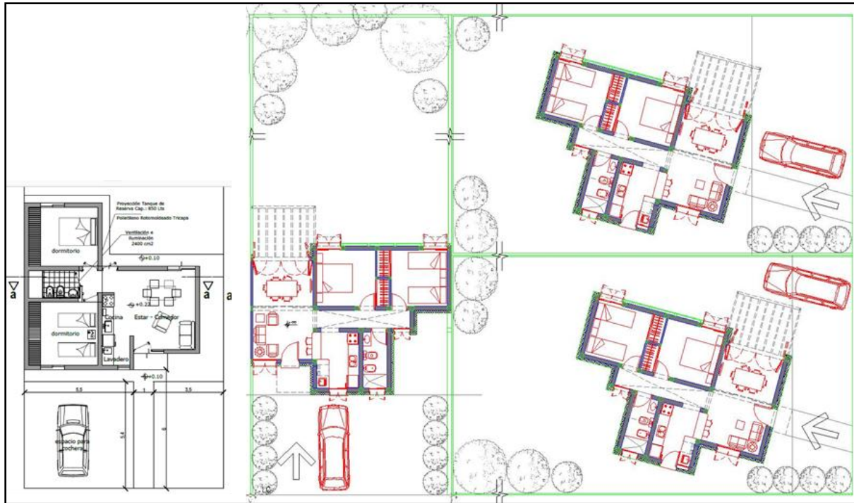
Figure 1: Left, IPV 2 bedrooms (with extension to 3 bedrooms) prototype. Center and right, INEAA two bedrooms (with extension to three bedrooms) bioclimatic prototype, with locations depending on lot orientation.
