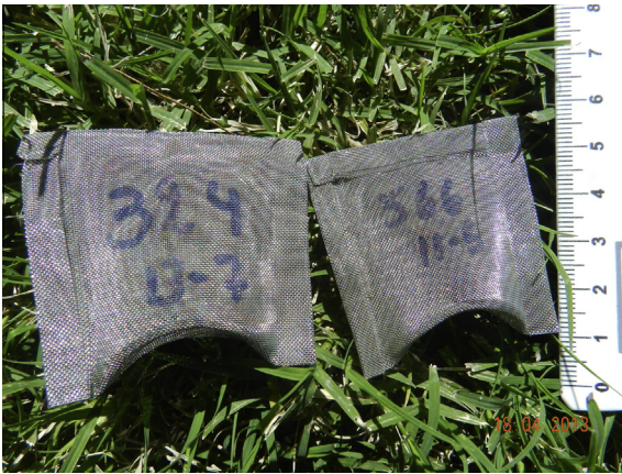
Fig. 2. Stainless steel wire mesh envelopes (5 × 5 cm) employed to expose the engorged females of Rhipicephalus (Boophilus) microplus in both forested and grassland areas.
