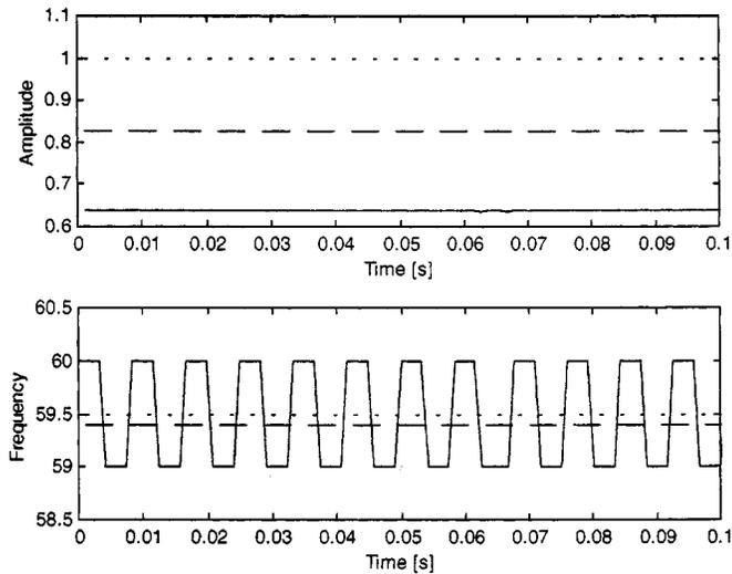
Fig. A. Estimated amplitude and frequency using DFT for the test signal of Fig. 1:  $T_w = 1$  s (solid),  $T_w = 3.33$  s (dashed) and  $T_w = 10$  s (dotted).
