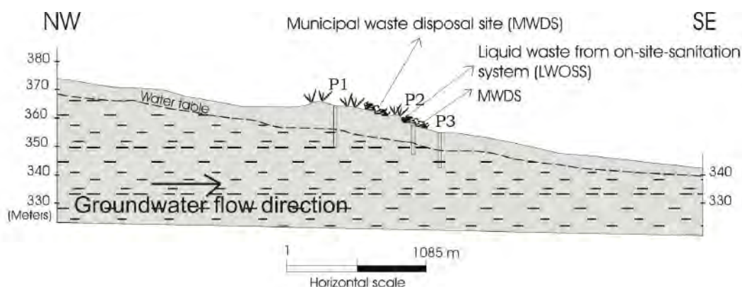
Figure 3. West - East hydrogeological cross-section through the MWDS along the line A-A` shown in Figure 2. P1, P2 and P3 are wells drilled on the disposal site area over a line flow.
