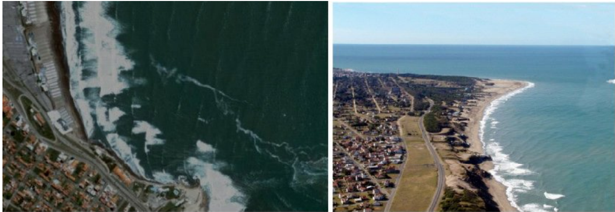
Figure 5. A. Punta Cantera operates as a headland or point break (in the sense of Scarfe et al., 2009) that causes wave diffraction with a peel angle improved for surfing; B. Pescadores Bank acts a natural reef causing wave refraction and protecting the tomobolo of Punta Mogotes. Waves from the south arrived obliquely and transport sand towards the tomobolo
