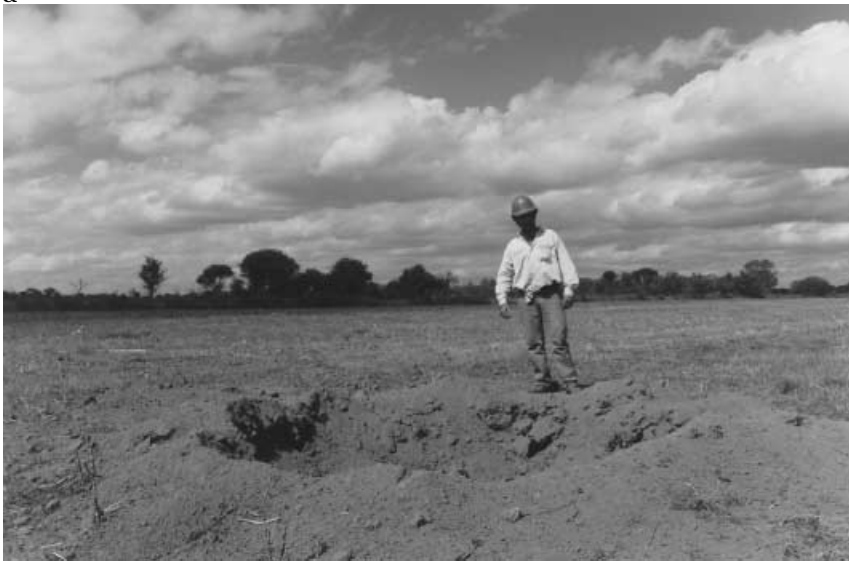
Fig. 8a,b. Craters obtained in two tests. a Superficial explosion crater; b underground explosion crater
