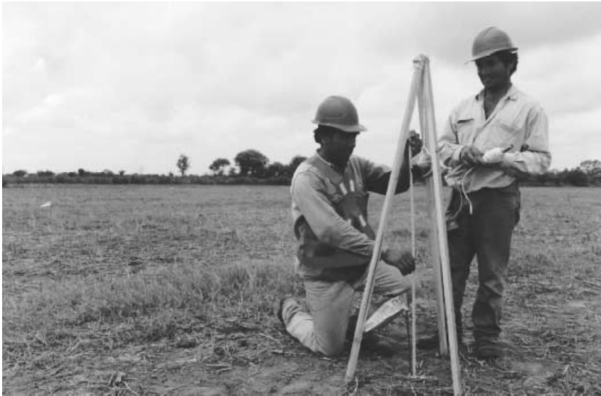
Fig. 3. Elevated-charge support system
