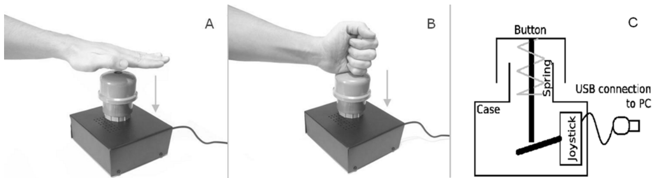
Figure 2. ACE: Response button and pre-assigned hand-shapes. (A) OH motor response during sentence comprehension task. (B) CH motor response during sentence comprehension task. (C) Custom-made response button. A commonly available USB joystick with analogue sticks was adapted to detect when a participant initiated a response. Reproduced with permission from [49].
