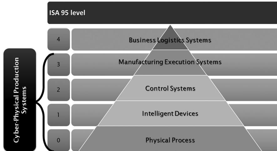
Figure 3. Levels of ANSI/ISA95 integrated into CPPS.
