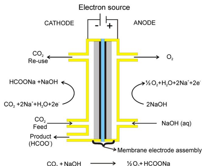
Fig. 1. Schematic representation of the CO<sub>2</sub> electroreduction in a fuel cell-like type of device.
