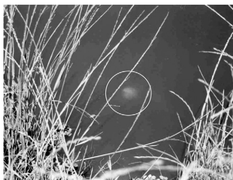
Fig. 3. Dialysis membrane bag placed in the stream.
