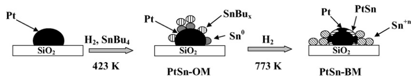
Scheme 1. Proposed images for PtSn-OM and PtSn-BM catalysts, based on characterization data and from Ref. [21].
