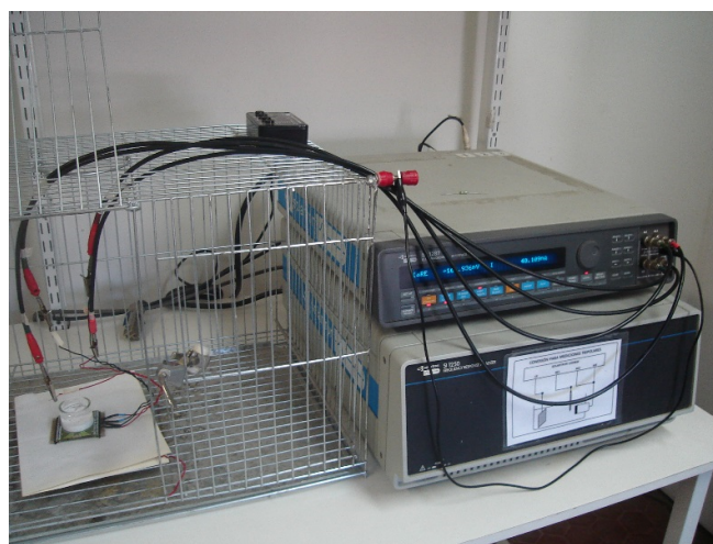
Fig. 12. Experimental setup. Solartron 1250/1287 system. At the left side of the picture the MEA platform is measured into a Faraday cage.
