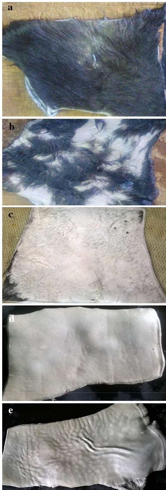
Fig. 1 Depilation effect on bovine hide. a Control with 0.6% (w/v) sodium sulfite without adding enzyme, b 0.025% (w/v) CpPL without sodium sulfite, c 0.025% (w/v) CpPL with 0.6% (w/v) sodium sulfite, d 0.05% (w/v) CpPL with 0.6% (w/v) sodium sulfite, e 0.10% (w/v) CpPL with 0.6% w/v sodium sulfite
