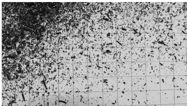
Fig. 2. Digital image of the as received rice husk ash (RHA), grid size is 5 mm.
