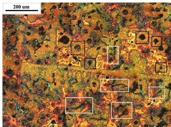
11 Zoom of microstructure. Black marked areas present graphite nodules enveloped by primary austenite. White marked areas show vermicular graphite particles in contact with LTF zones
