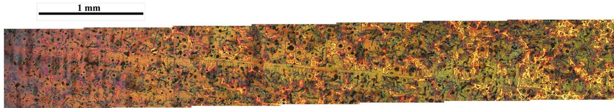
8 Microstructure of Melt B showing the dendritic structure of the austenite. Colour etched
