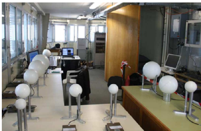
Fig. 2. HERMEIS neutron spectrometer located in the Pic-du-Midi station (altitude, latitude, and longitude are respectively equal to 2.885 km, 42° 55' N and 0° 08' E).
