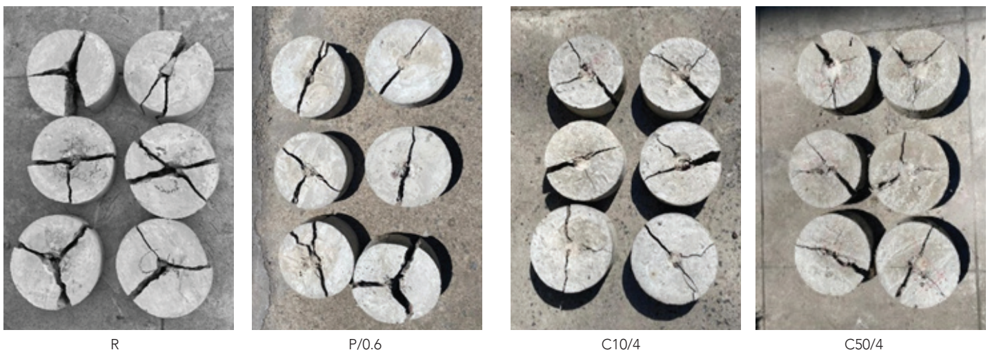
Figure 4: Images of some specimens after ACI 544 impact test
