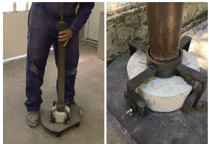
Figure 1: View of the used equipment for the ACI-544 impact test [30]
