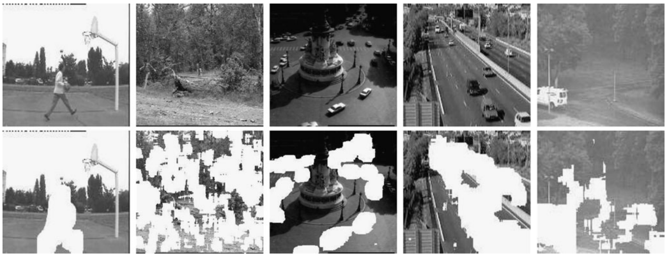
Fig. 3 Initial motion detection by computing the Number of False Alarms. The motion map is obtained by thresholding this quantity as explained in Veit et al. (2006). From left to right: the results are shown for the sequences Basketball, Forest, Traffic Circle, Route and Van.
