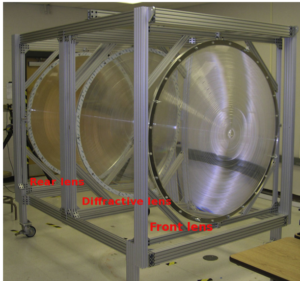
Fig. 4 The 1.5 m diameter three lens optics under test at MSFC
