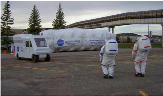
Figure 5. UND graduate students testing the integrated analog base systems. NDX-2 ATs, Electrical Rover and Inflatable Habitat can be seen from front to back.
