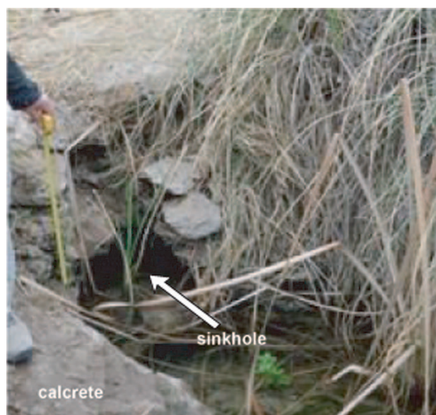
Fig. 4.- Sinkhole developed in calcrete near the Río Nuevo .
