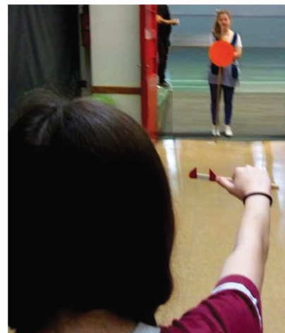
Figure 4. Measurement of the angle subtended by a 32 cm diameter cardboard disc at a distance of 6 m.
