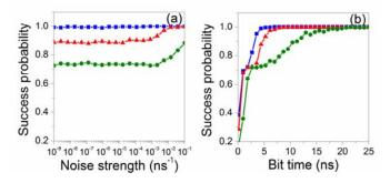
Fig. 8 (Color online) Success probability for y-polarized injection, as function of the noise strength (a) and bit time (b) using the criteria of 70/30 (squares), 80/20 (triangles), and 90/10 (circles). In (a) T=7 ns, in (b)  $D=10^{-2}$  ns<sup>-1</sup>; other parameters are as in Fig 6.
