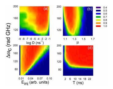
Fig. 5 (Color online) Success probability for x polarized injection, as a function of the detuning variation,  $\Delta\omega_c$ , and the noise strength, D (a); the pump current parameter,  $\mu$  (b); the injected field amplitude,  $E_{\rm inj}$  (c) and the bit time T (d). When the parameters do not vary, they are  $D=10^{-3}\,{\rm ns}^{-1}$ ,  $E_{\rm inj}=0.05$ ,  $\mu=1.2$ , T=4.5 ns; other parameters are indicated in the text.
