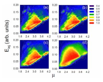
Fig. 9 (Color online) Success probability whit y polarized injection as a function of the pump current parameter,  $\mu$ , for noise strength:  $D=10^{-9}\,\mathrm{ns}^{-1}$  (a),  $10^{-5}\,\mathrm{ns}^{-1}$  (b),  $10^{-3}\,\mathrm{ns}^{-1}$ (c), and  $10^{-1}\,\mathrm{ns}^{-1}$ (d). T=5 ns and  $\Delta\omega_c=150$  rad GHz, other parameter as in Fig. 7.
